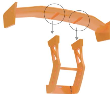
1. Bond the wing stay and wing plate together using instant adhesive.
