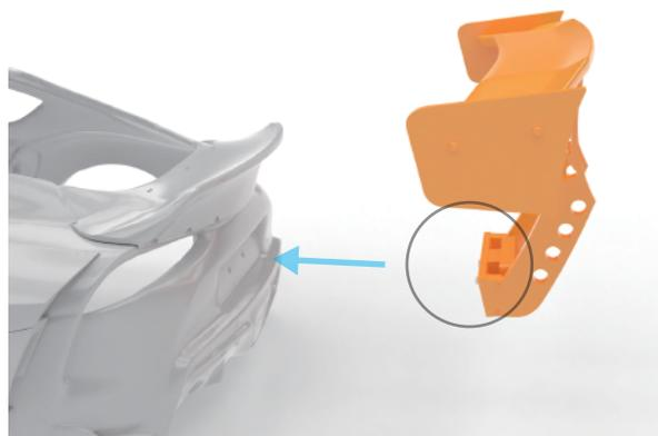
3. Fix the wing in place using instant adhesive at the Supra license plate position.
